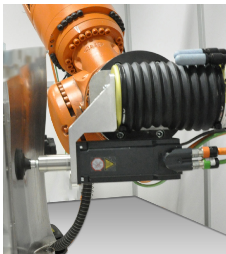
◄ Polishing machining grooves on titanium
